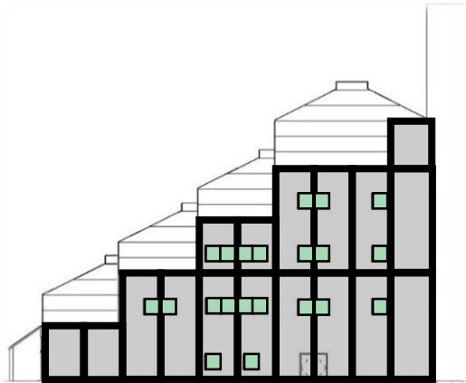
FIGURE CE.16: PRECAST PANEL EAST FAÇADE LAYOUT
